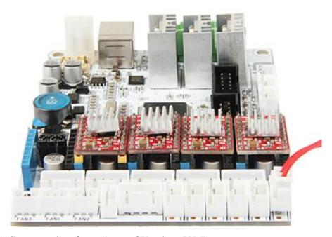
2) Connect wires for endstop of Y-axis at Y-Min.
