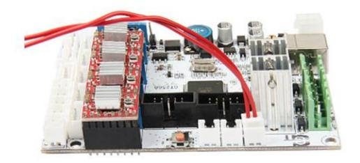
3) Connect wires for thermistor of extruder 2.
