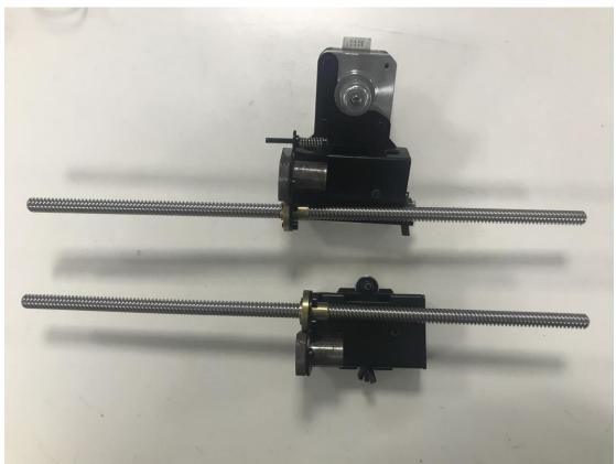
Step2. Plug the trapezoidal screw on the X motor end to the left coupling on the left bottom of the Z axis. Then thread the 320mm smooth rod into the linear bearing.
