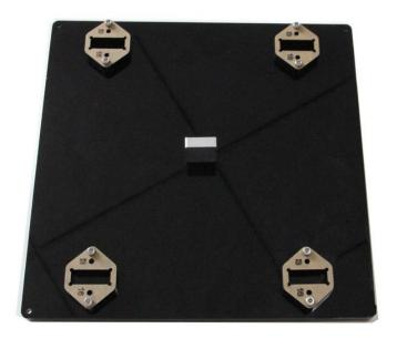
Step3. Get the build platform plate zip-tied to the 4 linear bearings of Y- Axis.
