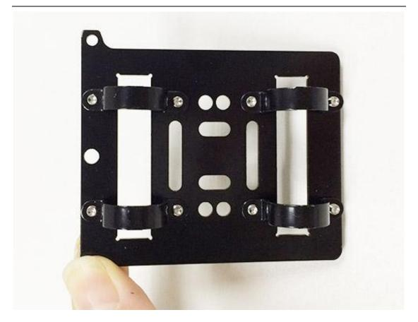
Insert the linear bearing into the slot and screw the bracket tightly.
