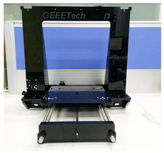
Step2. Screw up the main frame to the acrylic fender with 4 M3 x 20 screws. And screw up the M10 nuts.
