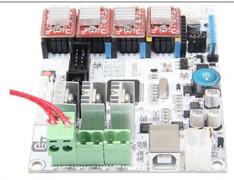
3) Connect heating wires for extruder 2.
