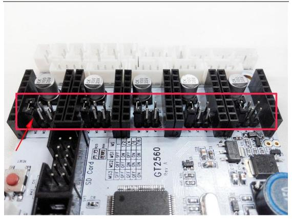
Step2. Plug the 4 A4988 into the stepper motor driver slot. Mind the directions of A4988.
