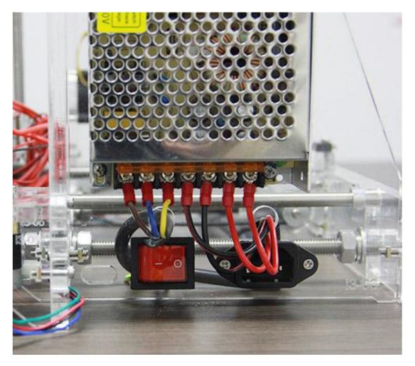
2) Pay attention to the switch on the right side of the PSU, there are two options of voltage: 110 V and 220V, choose according the standard in your country. As shown in the following picture. Remove the yellow paper; you can use some hard sticks to reach the switch.
