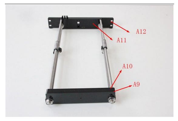
\* Tips: Try to keep the rods parallel and the four acrylic pieces parallel. The Y-axis must be a rectangle, that is the rods on both side should be parallel, so is the front and back plate. Otherwise it will cause obstruction for the belt later. You can use a Digital Caliper to measure.
