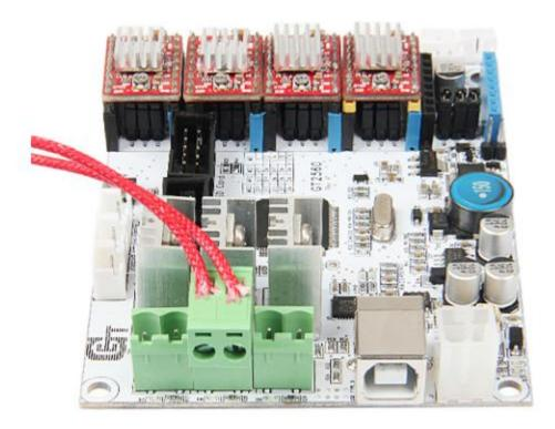
**Step4.** Connect wires for thermistor.
