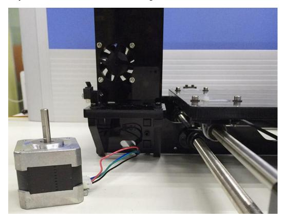
Step2. Screw up the motors with 4 M3 x 12 screws.
