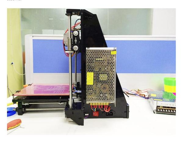
Step5. Now we can connect the wires to the PSU.
